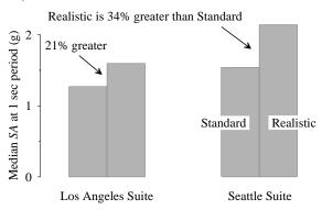
Figure 10. Standard and Realistic building model IDA results for median spectral acceleration at 1 s period causing collapse.
