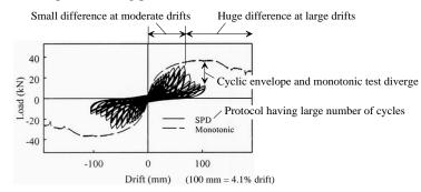
Figure 3. Results from experimental tests of identical plywood shear walls using two different loading protocols (adapted from Figure 6 in [8].
