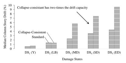
Figure 5. Drifts defining column damage states from laboratory tests using different loading protocols (standard and collapse-consistent). Data taken from Tables 3 and 8 of [10]. Y = onset of yielding, LB = onset of local buckling, MD = onset of moderate damage, SD = onset of severe damage, and ED = onset of excessive damage.
