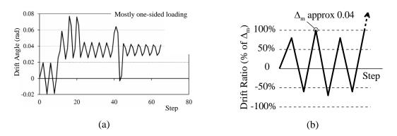
Figure 2. Loading protocols based on simulated building response. (a) Collapse-consistent protocol (adapted from Figure 8a in [5]), and (b) maximum considered earthquake (MCE) protocol based on median building response (adapted from Figure 18a in [6]).
