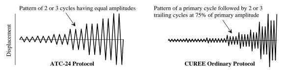
Figure 1. Representative standard loading protocols: ATC-24 [3] and CUREE ordinary [4].
